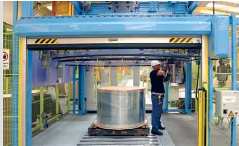
Wickelmaschine an der Coil-Pack-Station Wrapping machine at the coil packing station
