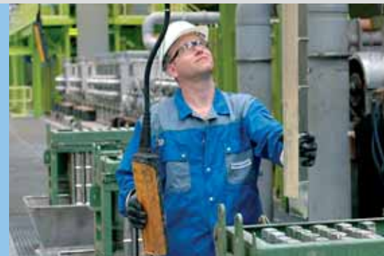
Zinnanodenwechsel Change of tin anodes
